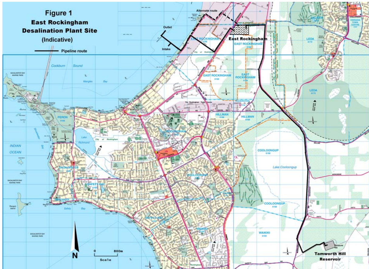
Figure 1: Indicative location of desalination plant and pipeline infrastructure at the East Rockingham site
