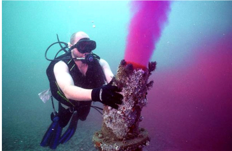
Figure 8.2 Desalination brine being ejected from a port on the Perth Seawater desalination Plant Diffuser (source: WA Newspapers). The brine was temporarily dyed red to show mixing with surrounding seawater.
