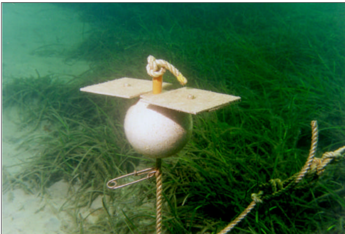
Figure 2-7 Periphyton collector on seabed
