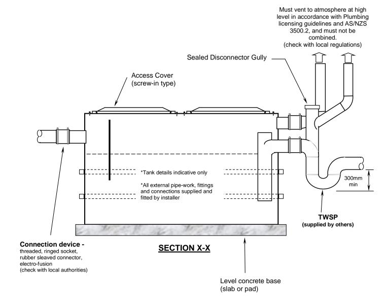
**NOTE:** Baffle and internal pipe configurations vary according to tank type capacity and/or customer requirements. The above drawing is indicative only. The installer must comply with local regulations when connecting a trade waste tank.
