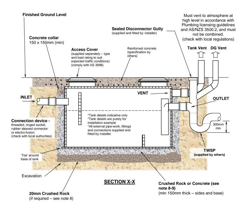
Note: Baffle and internal pipe configurations vary according to tank type, capacity and/or customer requirements.
