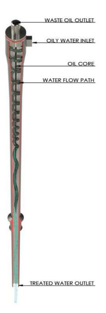
Cleanawater Hydrocyclone oil separators operate on the process where wastewater enters the cyclone chamber and is spun under extreme centrifugal forces up to 1000 times the force of gravity.
